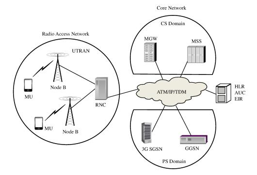
Figure 1.1: 3GPP UMTS Release 4 network architecture [1]
