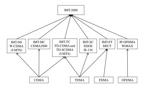
Figure 2.2: IMT-2000 radio interface standards [3]
