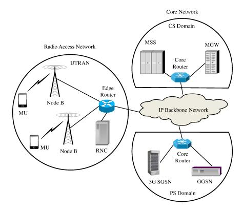
Figure 1.2: 3GPP UMTS all-IP Release 4 architecture
