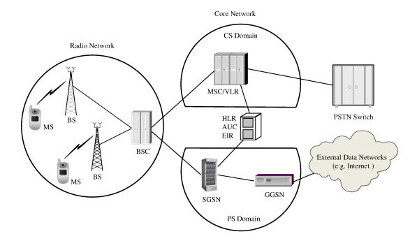
Figure 2.1: Architecture of 2.5G cellular networks
